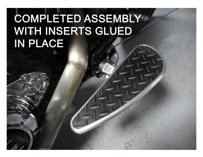
The clevises we supply are travel limited, so if the boards pivot up, they do not strike the exhaust on the right side, and the round engine cover on the left. The outside of the board is a little higher than the stock pegs, but if you ride agressively and scrape pegs, these may scrape too, and will only pivot up a fixed amount.
